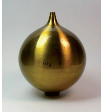
Helmholtz Resonator Source: Wikimedia License: CC BY-SA 2.5
